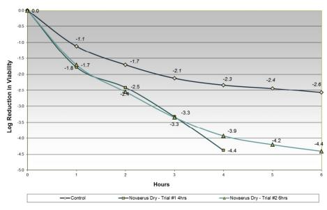
Figure 9: Aspergillus niger spores Control and NV900 trial LOG Reduction in Viable Concentration.
