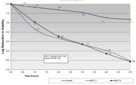
Figure 8: Bacteriophage MS2 Control and NV900 trial LOG Reduction in Viable Concentration.
