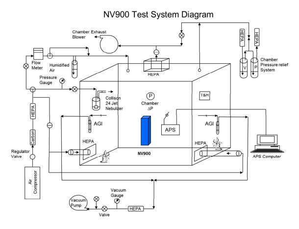
Figure 2: Bio-Aerosol Test Chamber Flow Diagram.
