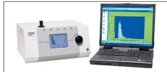
**Figure 4.** TSI Aerodynamic Particle Sizer (APS) model 3321 used to measure total particle concentration and particle size distribution of the challenge bioaerosol. Range 0.54-20.0  $\mu\text{m}$  aerodynamic diameter, with 1 particle/L detection limits.
