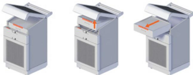
Markings on the filter to aid placement and correct orientation.
