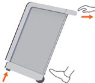
Stabilize the Defend 1050 at a comfortable angle, depending on the transporters individual height, where minimal pressure is exerted against the body to ensure stability.
