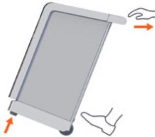
Stabilize the Defend I050 at a comfortable angle, depending on the transporters individual height, where minimal pressure is exerted against the body to ensure stability.
