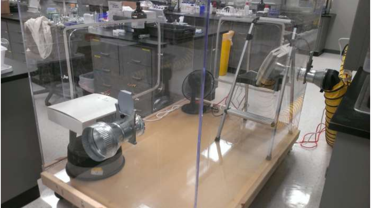
Figure 3: Plexiglas chamber for formaldehyde removal testing.
